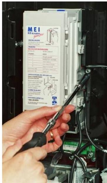
Figure 5-8: Securing the reader/DBV unit
