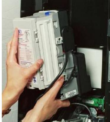
Figure 5-7: Mounting the reader unit
