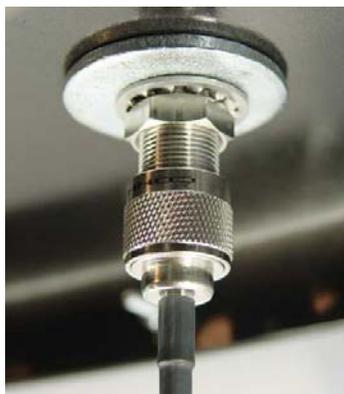
Figure 5-5: Attaching the antenna cable
